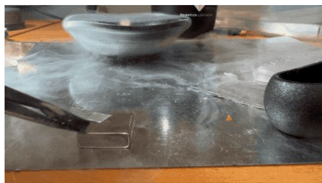
Flux pinning holds a levitator over a single magnet. Push it and it pushes back — the locking force students will measure in Chapter D.
