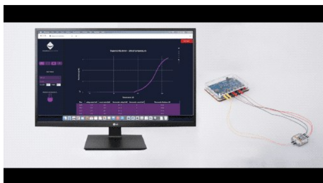
Experiment 2 in practice: the levitator's resistance thermometer logged on a laptop as it warms.
