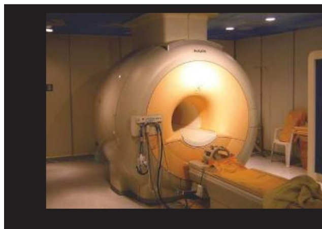
Figure 7. A conventional high-field MRI scanner, built around a superconducting magnet.
