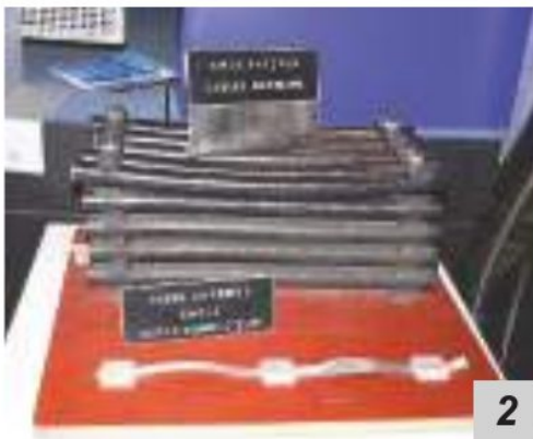
Figure 5. Conventional and high-temperature superconducting cables for 12,500 A at the Large Hadron Collider, CERN.
