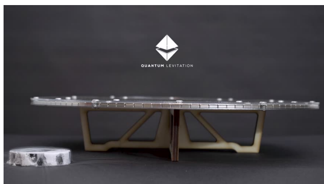
The circular maglev track: free along the rail, locked in every other direction.
