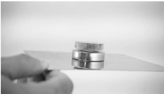
Tilt the plate and the levitator comes with it, locked to the field at every angle.
