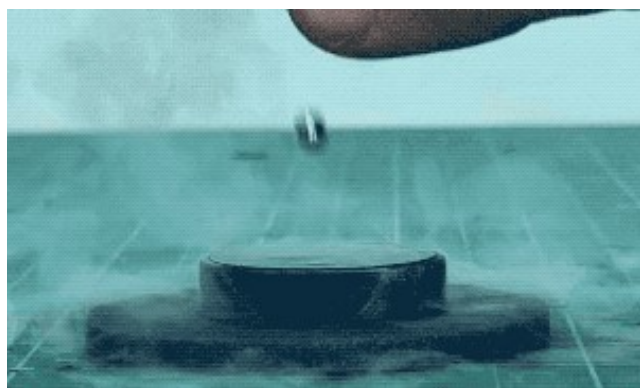
Activity 1: the magnet is pushed away whichever way round it is held — a perfect diamagnet does not care about polarity.
