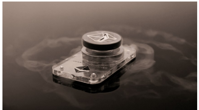
The near-frictionless bearing: locked radially, free to spin around the ring magnet's symmetry axis.
