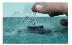
Conclusions: In the Meissner state the superconductor is a perfect diamagnet - it has a magnetization opposite in sign and equal in magnitude to the surrounding magnetic field. It therefore exhibits an unstable magnetic repulsion, like two repelling magnets.
