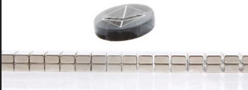
**Experiment:** Position the flexible track on a firm surface, either on its wide face or on its side. Soak the levitator in liquid nitrogen. Using the tweezers take the levitator and lock it on the track. See how it moves smoothly along the track. Try changing the levitation height, see how it reacts.
