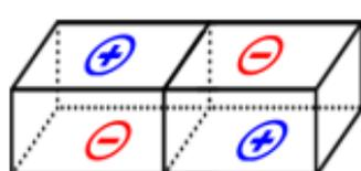
2. Attach the pair above or below the stain-less steel track.
